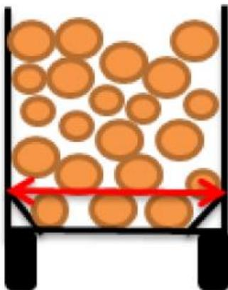
Figure 2. Measurement point for measuring lower bank width.
