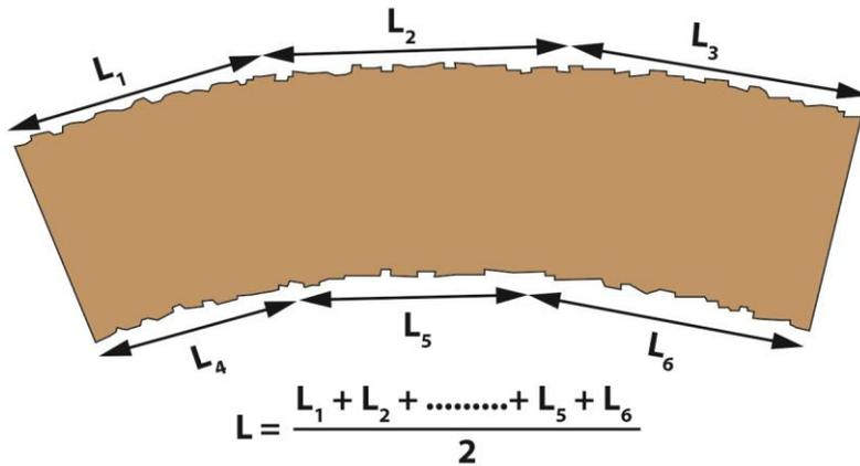
Figure 4. Measuring the length of a crooked stack.
