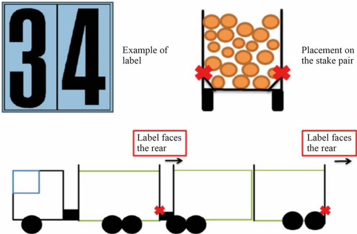
Figure 3. Examples of labels showing lower bank width, and how they should be placed on the vehicle and trailer. Before the labels are applied, the surface should be cleaned thoroughly to ensure that the labels adhere properly and remain in place.
