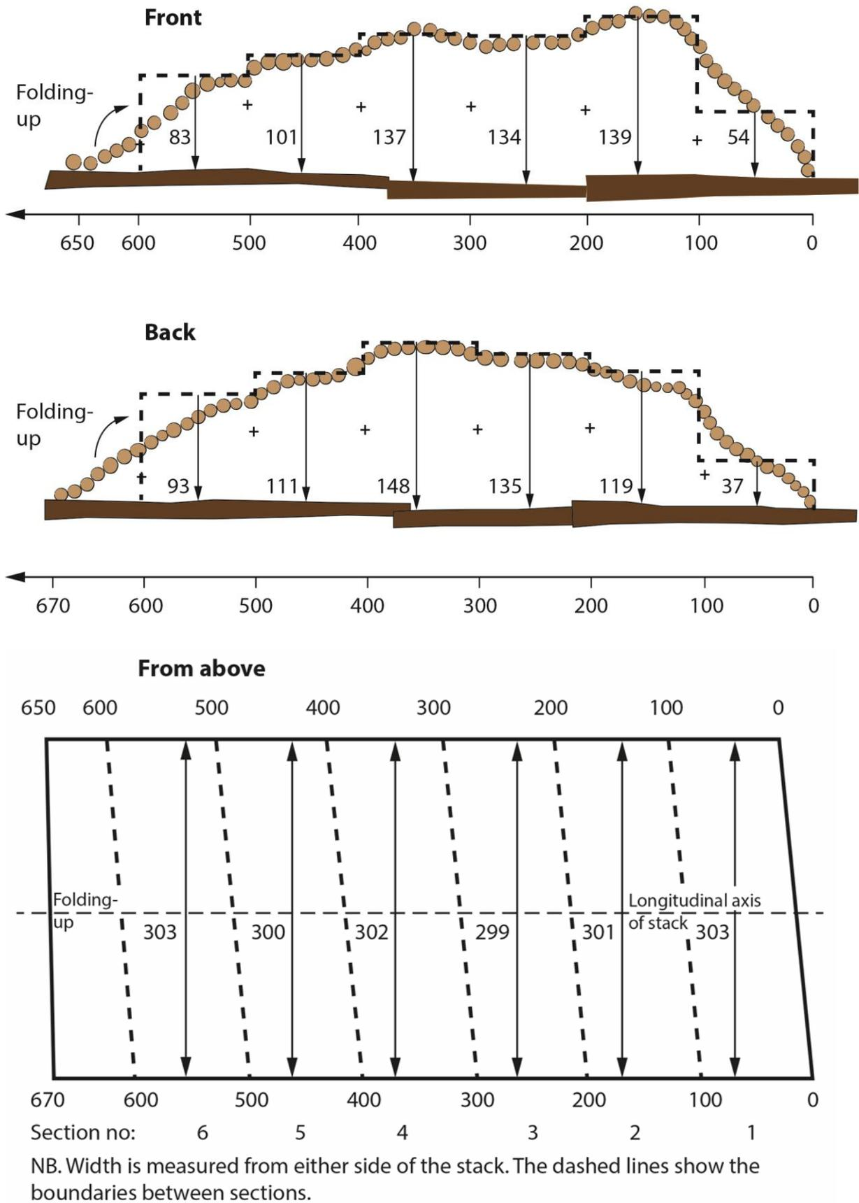
Figure 5. Measuring the volume of a stack.
