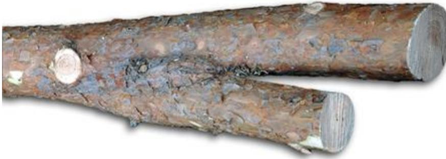
Figure 2. Open fork – air between fork limb and the main stem.
